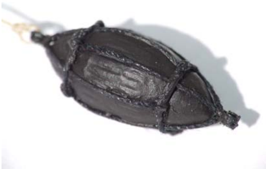
Buoy. The finished nun buoy with a rope tied to the eye at one end
