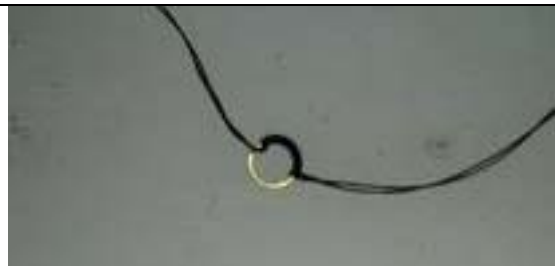
Anchor ring 2. The thread is wrapped around one half of the ring
