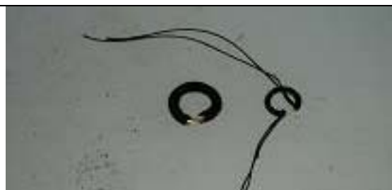
Anchor ring 4. Both sizes of anchor ring with puddening
