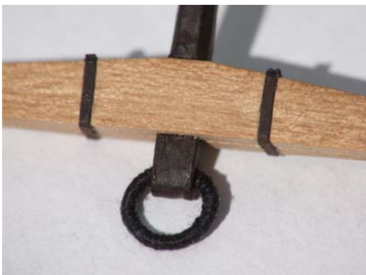
Anchor 12cwt. The iron bands have been wrapped around the stock and the ring has its puddening of thread
