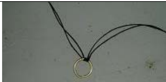
Anchor ring 1. A couple of turns of doubled thread are laid around the ring and glued
