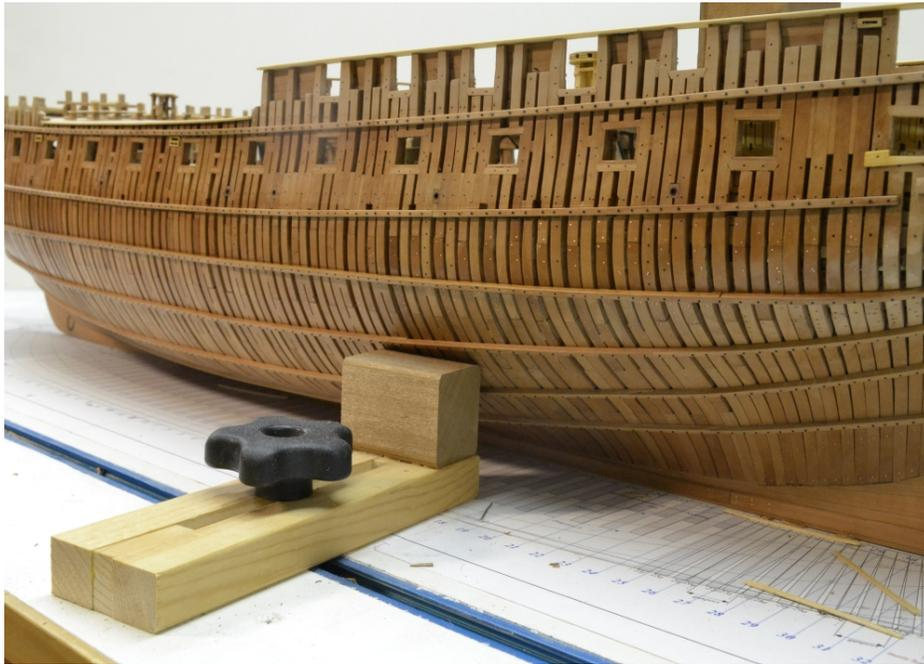
The clamping base was made from pine strips. The support block was made of another soft wood, in this case white cedar, but any soft wood will suffice. The top inside corner of the block should be rounded. I made four of these.
