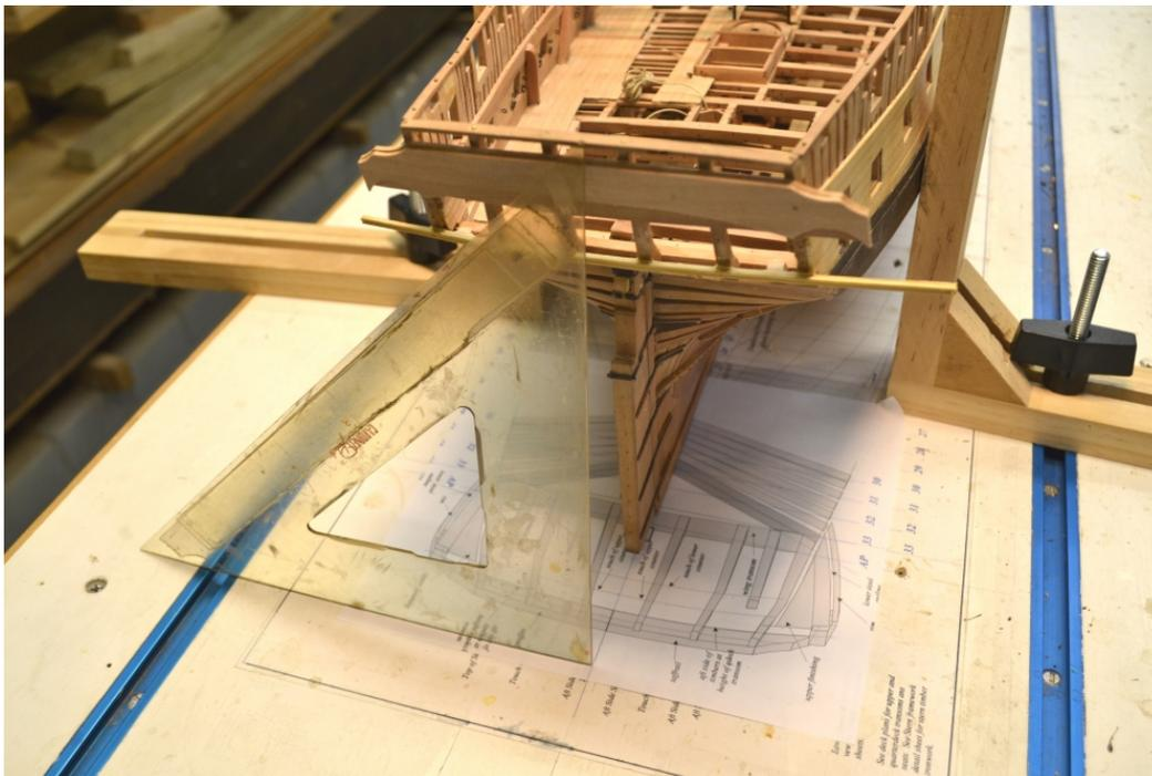
With the clamps in position, a triangle is being used to center the top of the stern. Whenever the model is turned upright, repositioned or when the clamped squares are moved, this process should be repeated – fore and aft. It may be tempting not to do it if no precision construction is being done, but I recommend doing it every time to get in the habit. It is also possible that you may
