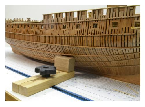
The clamping base was made from pine strips. The support block was made of another soft wood, in this case white cedar, but any soft wood will suffice. The top inside corner of the block should be rounded. I made four of these.
