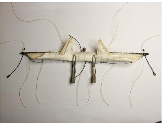
Now the gaskets at the centre of the sail are coiled around the sail: at the back the gasket hangs down, at the front it is pulled up and then over the yard. The second turn brings
