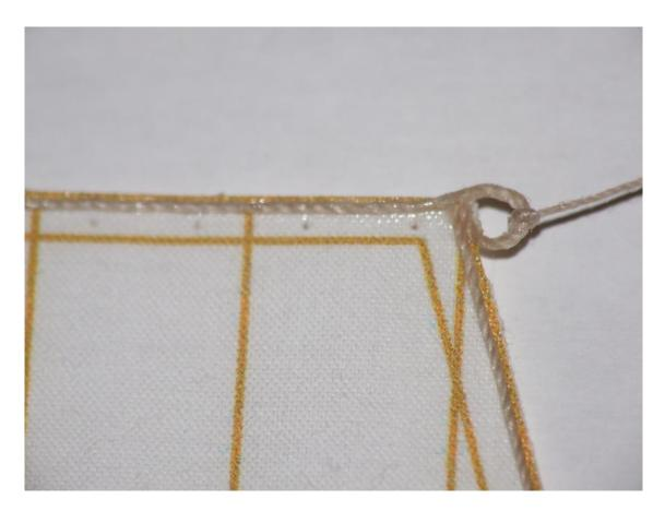
The sail is attached (bent) to the yard in a reasonably authentic way. I first tacked it in place with a couple of clips (this part is not authentic) so that the top edge of the sail is near the top of the yard: according to most references the sail does not hang under the yard. The bolt rope is at the back of the sail.
