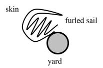
Gasket ropes are used to hold the furled sail in place. On the topsail one is tied to the yard at each end, through the earring cringle, one is half way along each yard and two (known as the bunt gaskets) near the centre of the yard. The gasket is wound around the sail and yard for somewhere between four and seven turns with the last few turns being closer together. The loose end is not tied with some fiendishly complicated knot but is simply wrapped round and round the last few turns.
