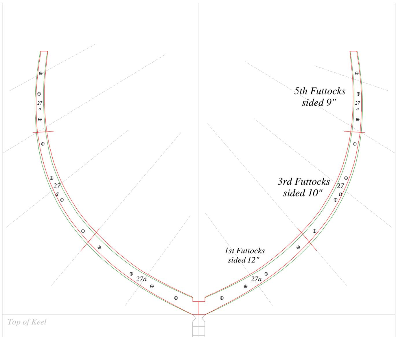
⊕ indicates bolt center for drilling - not size.
