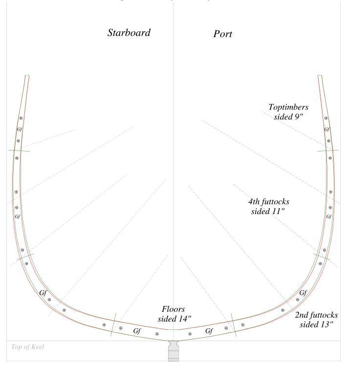
• indicates bolt center for drilling - not size. (Frame bolts 1" iron - not headed) Rev.3/11/16
