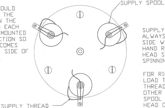
SUPPLY THREAD SHOULD ALWAYS FEED FROM THIS SIDE WHEN DOING LEFT HAND ROPE AND THE HEAD SHOULD BE SPINNING CCW.
