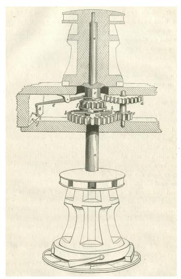
The annexed figure shews the two capstans, as detached from each other. a a the shaft of the lower capstan: it rises through the deck, and into the upper capvol. XLIX.
