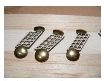
Complete this activity before fitting the windows to the ship/part. Pin the frames down over a sheet of release tape (Sellotape or similar). As the glazing resin is very liquid, to stop it running out I put a drop of Golden self levelling gel in each opening. This forms a lining and seals each cell. After allowing 12 hours to cure, ensure there is no dust in the cells, and then fill each with a drop of 'Solid Water'. A touch of a flat blade on the top of each
