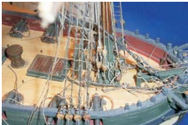
Neb has yet to finish rigging the fore and main back stays nor has he tied anything down permanently yet. The tackles showing at the base of the mast are the jeer and truss tackles.
