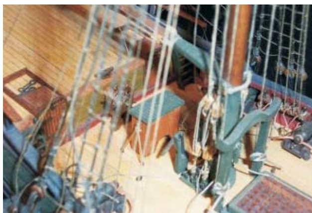
Note the pumps just aft of the mast. Just aft of them is the binnacle which is a 'sideboard' type that is lashed to the deck through eye bolts.
