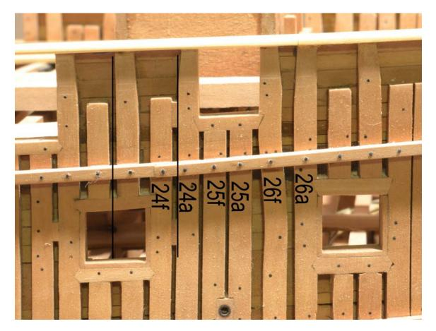
This is the only cant frame requiring this. For the two aftermost carronade ports, precise locations are shown for the upper frames on drawing 2 and 2B. These locations are used to set the cant frames so the carronade ports will be sized correctly.
