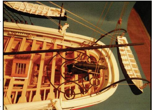
Parrott rifles. These latter two pieces are mounted at the bow and stern on concentric photo-etched brass tracks, and are another unique aspect of warship design during this period.
