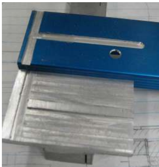
Figure 9. Press-fit slots on joint between fence and guide bar.
