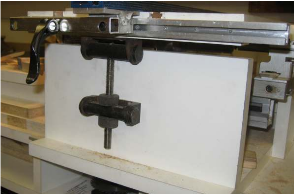
Figure 6. Table height adjustment and details of the fence.
