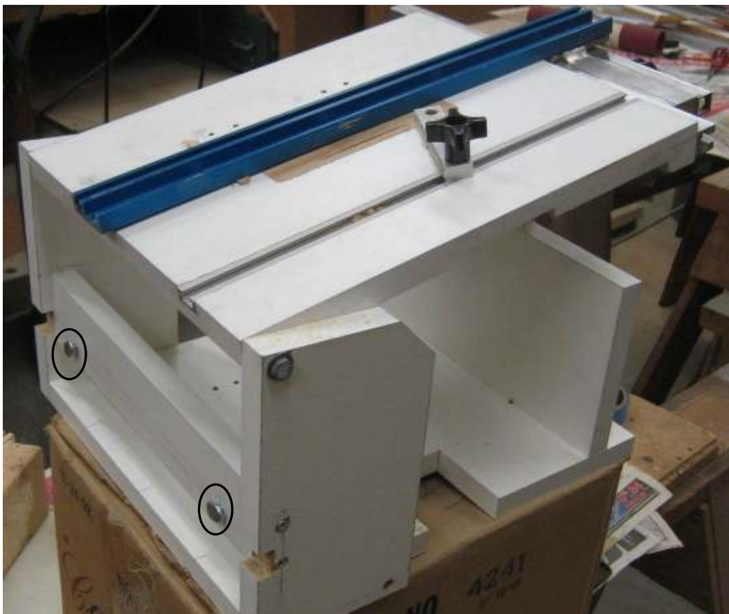
Figure 4. Table saw module. T-bolts (circled) hold base to T-slot at the back of the lathe base
