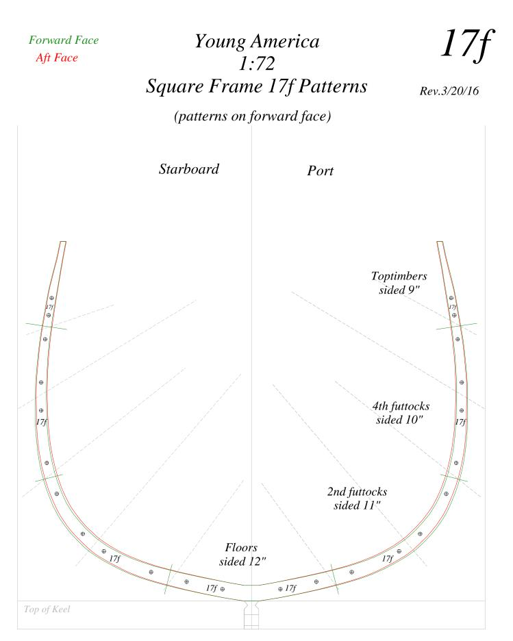
• indicates bolt center for drilling - not size. (Frame bolts 1" iron - not headed)
