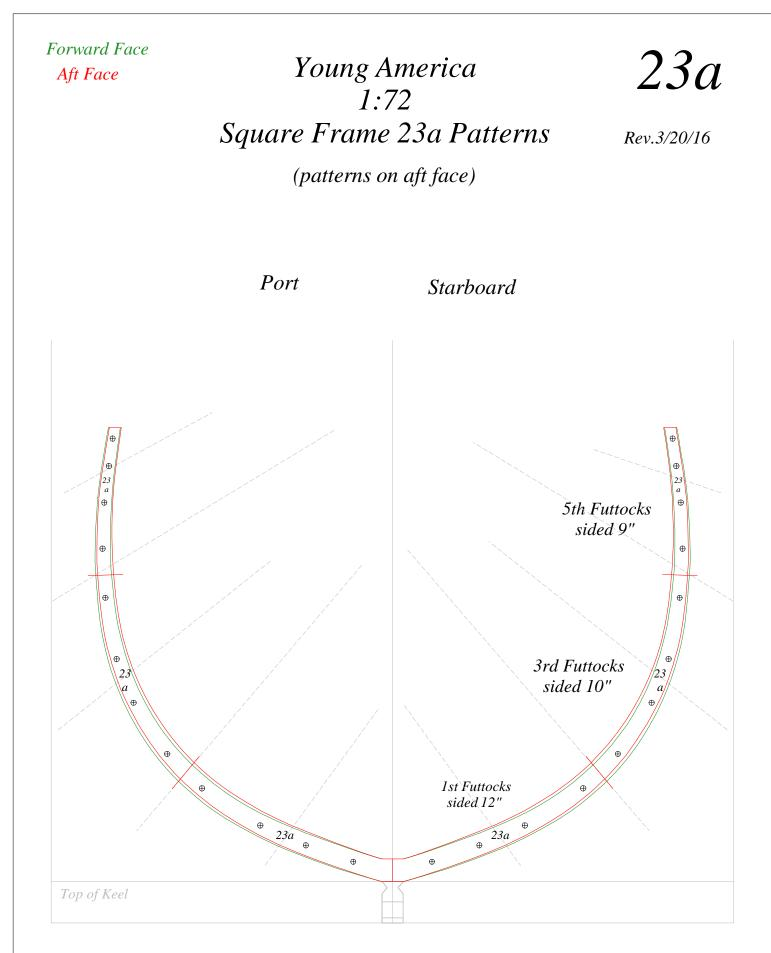
indicates bolt center for drilling - not size.
