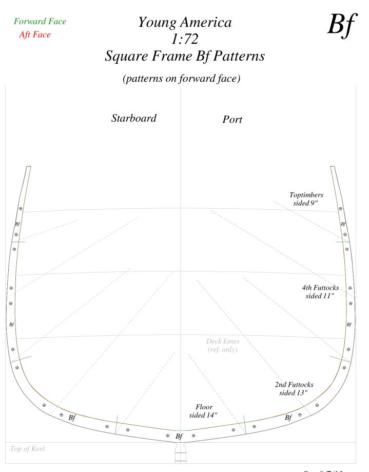
indicates bolt center for drilling - not size.
