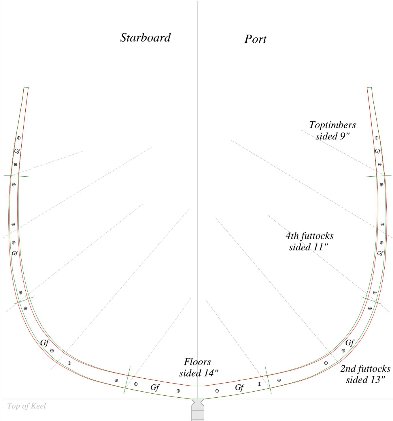
⊕ indicates bolt center for drilling - not size.
