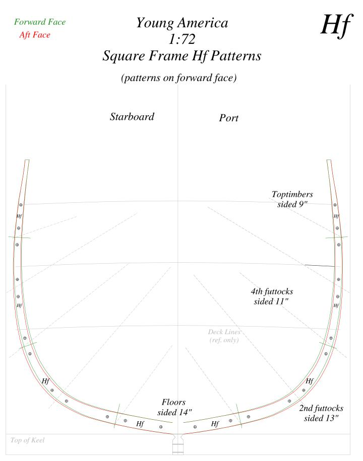
• indicates bolt center for drilling - not size. (Frame bolts 1" iron - not headed) Rev.3/11/16
