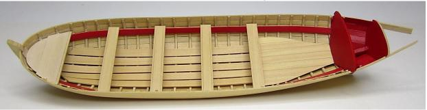
sure it fit properly, I cut the platform to shape and glued it into position. Then I glued the first thwart on the model. The thwart actually butts against the platform and sits flush with it. Also note in the photo posted on the previous page that the seatback and helmsman area were painted red before the thwarts were added.
