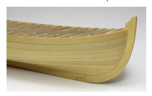
be consistent at all. In all probability, it will be wider than 3/16" (especially at mid-ship). A wider 1/4" x 1/32" strip is provided in the kit for this purpose. Carefully shape this final plank to fit the opening on your hull. Because it is in the middle of the hull where it begins curving towards the keel, the wider plank won't be noticeable when viewing the model from port or starboard.
