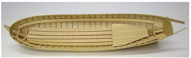
one down the center of the false keel. Then add two on each side of that initial strip.
