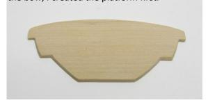
The platform was made by gluing three small lengths of 5/16" x 1/16" boxwood strips together edge-wise. No need to simulate the caulking this time since the platform will be painted. I created a card template to create the shape for the platform just like I discussed for other aspects of the build earlier. Once I was
