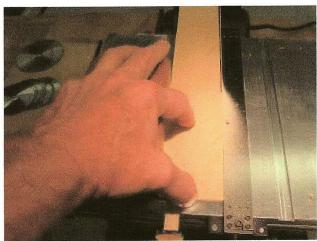
Initially I just had my fingers up on the block. Over time I've found the above hand position is more comfortable for me. I do not recommend this nor accept any liability for doing it this way, but that is what I do. Small finger is on outside of block and using it in combination with my palm is how I apply a little pressure. The above boxwood sheet is 1/8" thick and I am milling 1/32" x 1/8" strips.
