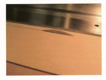
The above strips were milled for a customer order. As I am milling every 25 strips and if I switch to a new piece of sheet stock, I always mic them at each end and a couple spots in between. In the above picture the strips varied by .0005" over their length and were consistent from strip to strip. Most times the variance will be +/- .0015.
