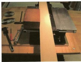
Block of wood is: 2" thick - Keeps my hand above the table and blade
