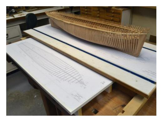
This photo was taken last November, shortly after deciding to incorporate a POB version in the book. The shipway is much simpler – no T-tracks and made from a melamine coated particle board shelf. The shipway plan is also simpler and geared to setting bulkheads instead of square, half and cant frames.
