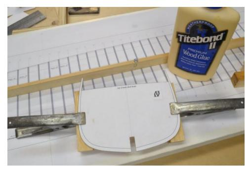
Most frames have four of these that fill the space between the plywood bulkheads. When faired to the outsides of the bulkheads, the spacers will provide a smooth, flat planking surface as well as great strength to the assembly. More on these spacers in the next part.
