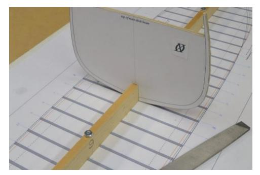
The bulkhead is cut from 3/32", aircraft grade plywood, from the pattern shown. The pattern is an early version – note the pasted-on ID. Other detail was later added to the final patterns. The bulkhead includes the toptimbers. These were sided 9" (3/32" at 1:96). The high quality plywood will allow these to be finish sanded and painted, eliminating the need for separate toptimbers.
