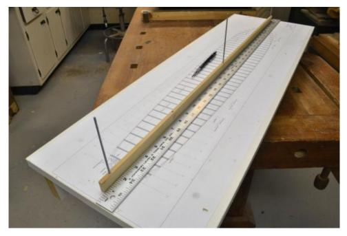
The spine is not a keel and does not replace the keel. A fully detailed keel assembly will be fit under this later. This is merely a device on which to align bulkheads. It is thick enough for that purpose and initially extends well beyond the hull.
