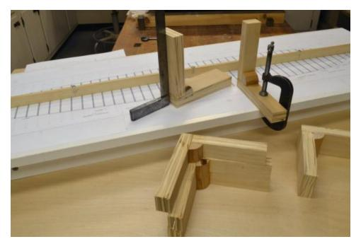
The picture also shows simple, homemade squares that can be clamped to the shipway as shown.
