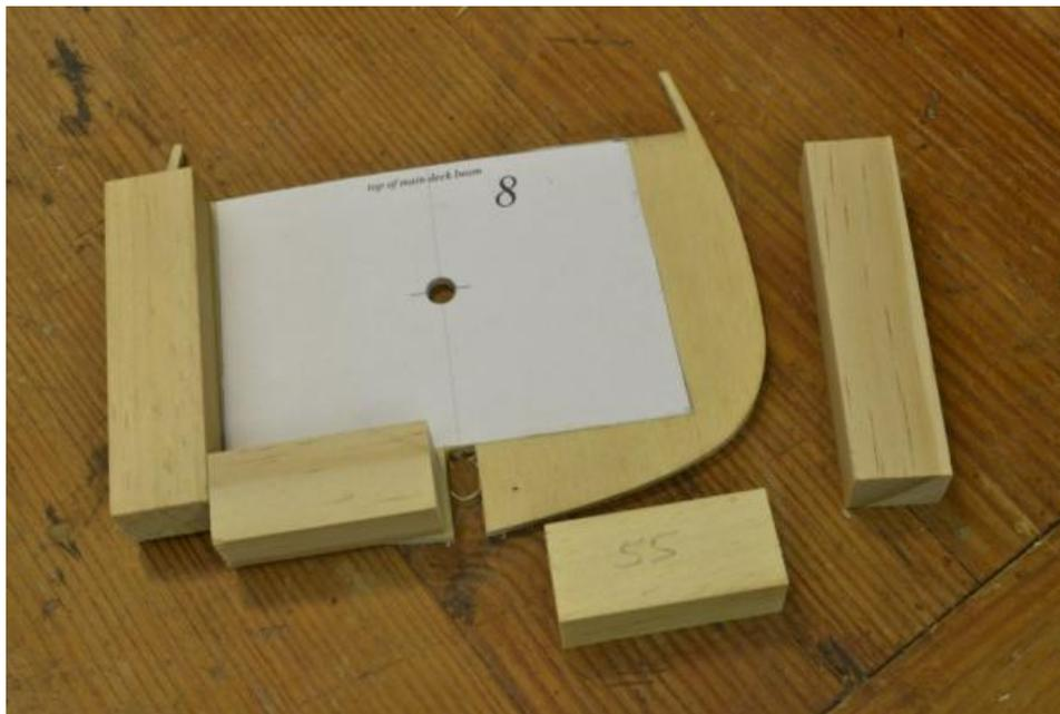
The spacers in this picture were cut to a width of 55" – marked on one of the loose pieces. Station spacing in this area is 64". Subtracting the 9" plywood thickness leaves 55". As mentioned before, 9" plywood was used because that is the siding of the integral toptimbers.
