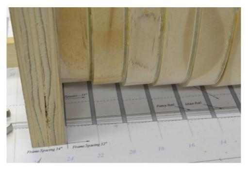
Note that the station lines on the shipway plan align with the plywood bulkhead at its maximum breadth. When the hull is faired by removing the excess and smoothing the line to over the plywood sections, the hull shape will be precise.
