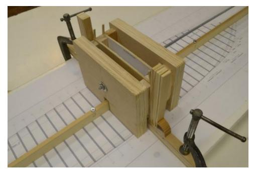
The squares are used to align the frame to the maximum breadth line on the shipway plan. The nut on the threaded rod is then tightened to secure the glued joint. The next picture shows more bulkheads added - one at a time.
