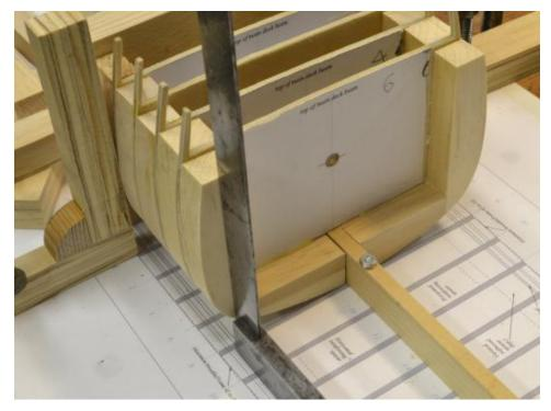
The bolt in this picture is on frame line 9. The picture was taken before bulkhead 8 was installed (and before the numbers on the patterns were moved toward the center). The next picture shows this nut encased.
