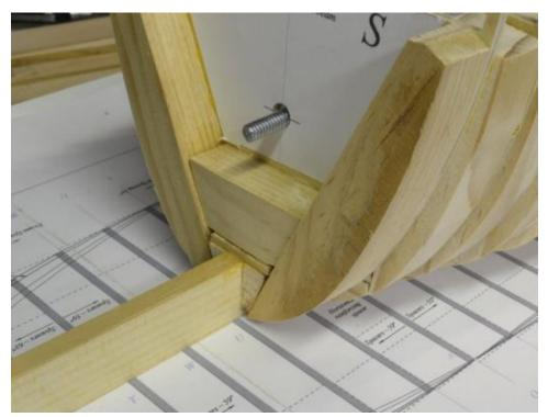
Although each of the three installations of these is slightly different, in every case there is a cap to hold in the nut and to act as a stop when the stud bolt is threaded in. All the parts are glued to the plywood as well as the side spacers, the assemblies are very strong. Next the mast steps.
