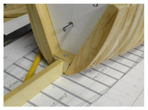
In this case tow triangular blocks were glued to the spine and the strip encasing the nut is glued to it. In the next picture the assembly is capped with another fitted block.
