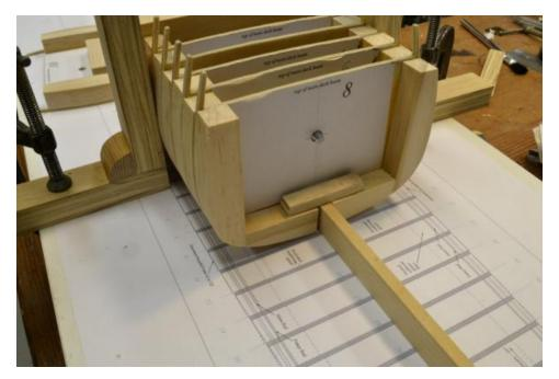
The nut is encased in the lower of the two hardwood strips glued to the top of the horizontal spacers. The lower strip is shown in the next picture, before the hole was filed to fit the nut.
