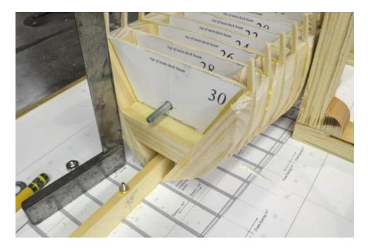
The next picture shows the hull framing well advanced. The squares clamped to the shipway are important. They keep the hull plumbed to prevent twisting as new bulkheads are added.
