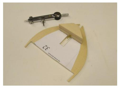
The holes for the brass pins need to be precisely located, hence the dividers. The drawings show these locations at the height of the spacer blocks. The pins are slightly raked – roughly matching the mast rake.
