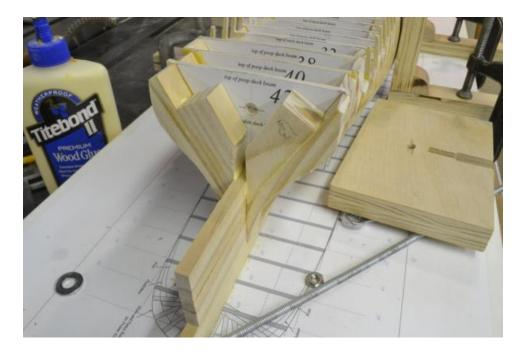
Also, in this picture, additional spacers have been inserted inside the outer ones to maintain a solid hull surface where the lines converge sharply at the stern.
