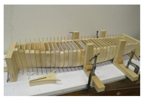
The last picture shows the hull framed back to bulkhead 42. At the ends, the central spine needs to be built up with additional tiers to form the deadwood as the hull narrows.
