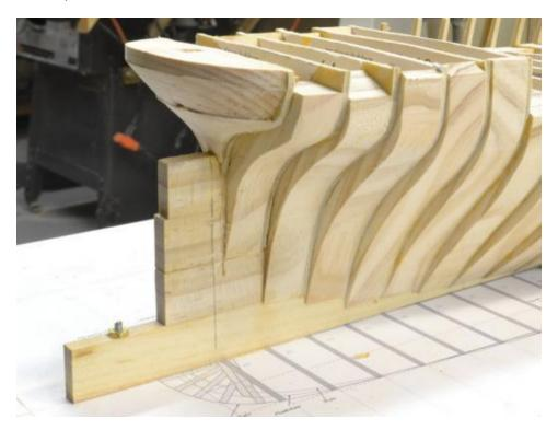
The pencil line shown was drawn using a template. This end of the hull is now ready for fairing – or will be when the excess spine material is removed. But first the bow will need to be constructed – in the next part.
