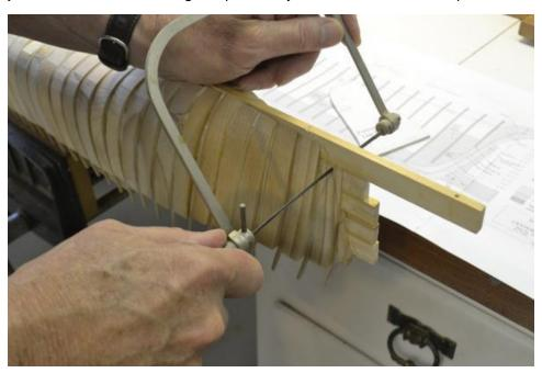
The spine aft of the post was also removed by cutting on a line marked from a stern template. Both these cuts are rough at this stage.
