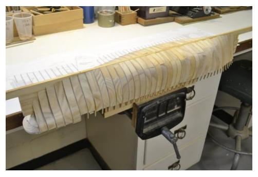
Removal of the excess spine was the first of these steps. In the next picture a coping saw is being used to cut just outside of the bearding line previously marked on the forward part of the hull.
