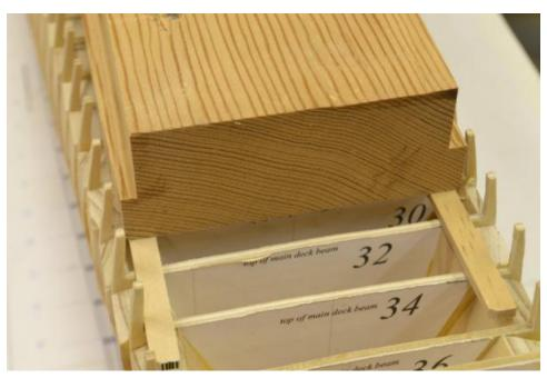
Two strips of wood were used to keep the block from rocking on the round up of the deck. The next picture shows the hull securely clamped in a bench level woodworking vise ready for the next steps.
