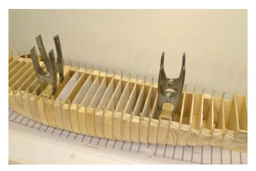
The wood block was rabbeted along the sides as shown below to keep the toptimbers clear of the vise jaws.
