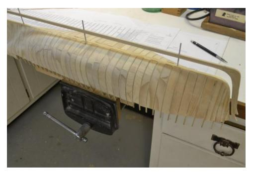
With the stem/keel still unglued, the hull was bolted down on the shipway and plumbed so the stem could be centered. The next picture shows the hull being marked to show the sides of the stem.
