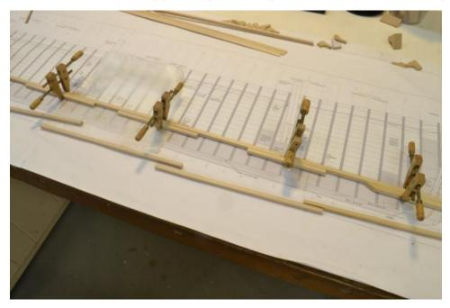
The pieces of the lower tier are shown below the glued assembly before their joints were cut. In the next picture the keel assembly with the two tiers and the shoe has been glued to the false stem assembly and the stem is being glued into the angle between the two assemblies.
