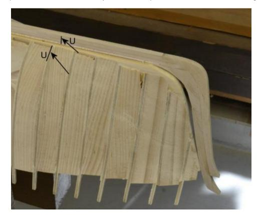
In the next picture the stem/keel assembly has been fit up to the inverted hull for final fitting.
