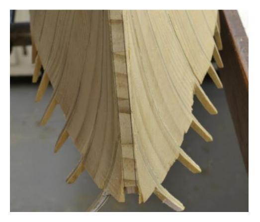
The stem was next refitted and aligned to the marks so locating pin holes could be drilled as shown in the next picture.
