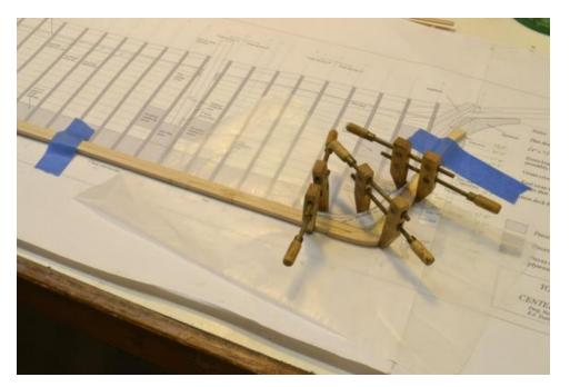
The stem and keel were taped to the drawing to preserve alignment when fitting and gluing the stem into place. The stem provided enough reinforcement to prevent to stem shape from distorting in the next steps.
