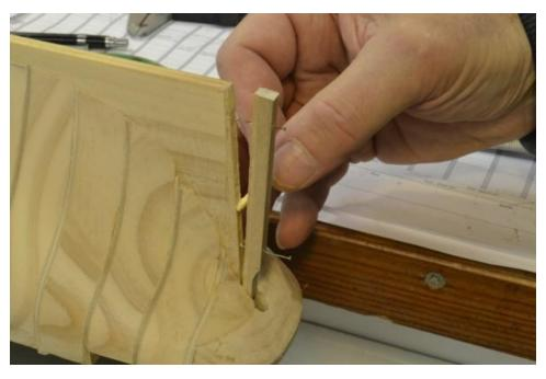
The keel assembly rabbet was extended only back to the inner line of the post, as shown below, deferring final rabbeting until after assembly.
