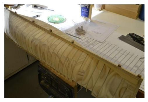
The hold down bolts were in position for the gluing/clamping, but were removed to avoid them being glued in.
