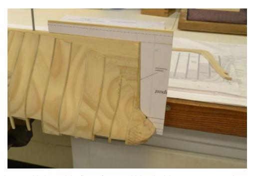
The filler piece provided a straight, flat surface on which to bed the sternpost – assuring a good joint and clean surface for shaping the deadwood into the sternpost rabbet. In the next picture, with the hull plumbed, the sternpost centerline is being marked on the filler.
