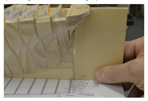
The template is aligned at station 50. The picture shows the need for a filler piece. In the next picture the hull has been cut back for the filler, it has been installed, and the hull is being checked again with a different template.
