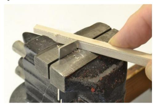
The rabbet was formed on both sides in this way – all the way to the bottom of the post up to the intersection with the hull at the top. In the next picture the post is being glued to the hull.
