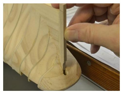
Holes for locating pins were drilled with the post in position. The bottom of the post was then cut off flush with the bottom of the hull. In the next picture the sternpost rabbet is being scraped out using the vise as a guide.
