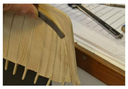
At the stem the area outside of the bearding line must be further pared back smoothly into the stem rabbet that was cut before assembly. In the next picture that is being done with a shallow gouge.
