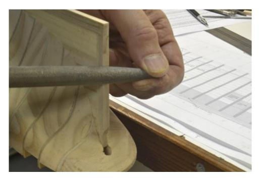
The post bevels allowed the rudder to swing over its full arc without being obstructed by the post. After this work, the lower hull was ready to be planked.
