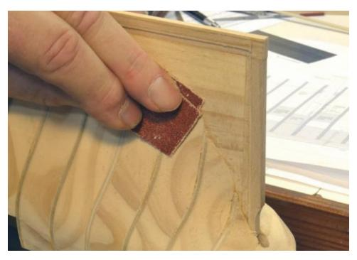
The final sanding of the hull was done using 120-grit paper.
