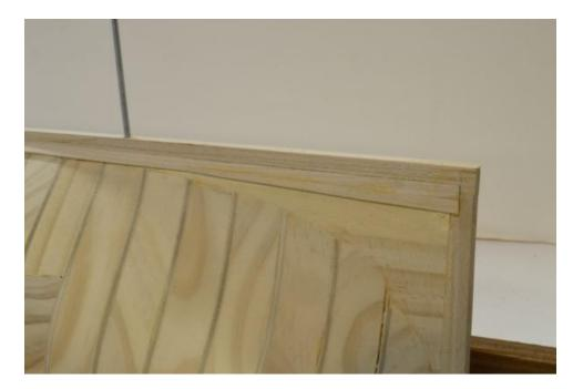
I did not use dark glue for any of the hull planking since the intention is to paint and sheath the hull later. Hard maple was used for all of this planking.
