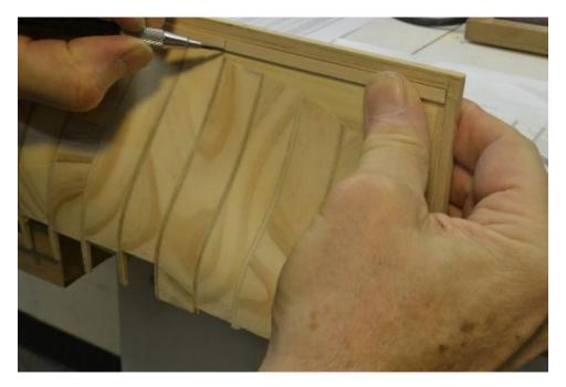
In the next picture the strake was cut to receive the second section and is being held in place to check the final fit.
