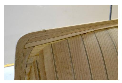
In this picture, it can be seen that the line of the rabbet runs just aft of the joint line between the stem and false stem.
