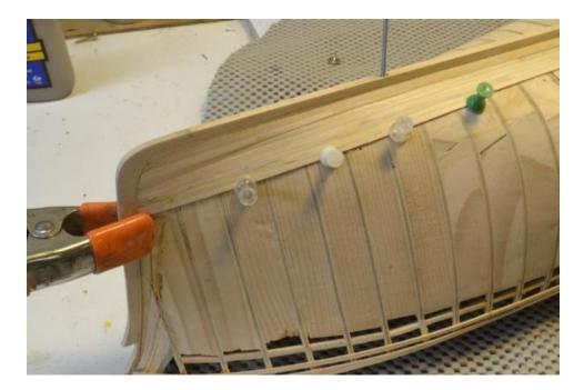
The clamp shown at the stem applies quite a lot of pressure to hold the "hooding ends" tight in the rabbet.
