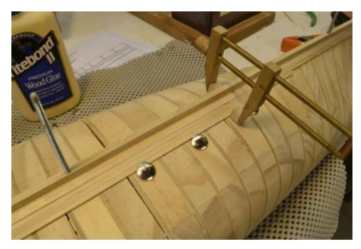
Drawing pins also work well in the pine substructure as shown in the next picture, but in general I used thumb tacks. The type with plastic covered heads are best. With the tapping in and prying out the attrition rate on thumb tacks was high.
