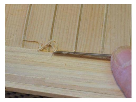
In the next picture the partial strake has been fitted and is, itself, being marked for another cut in strake.
