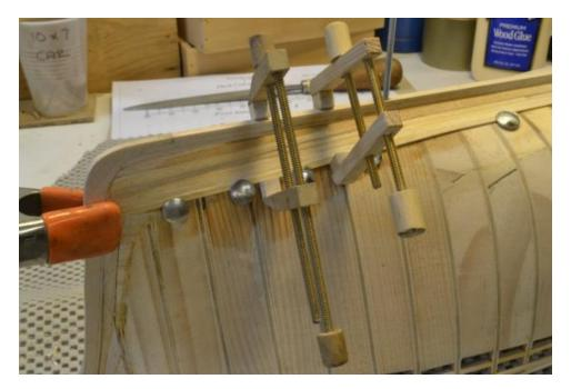
I used hard maple for all this planking. The picture shows typical clamping. Thumb tacks proved very useful and easy to use on this work. The soft pine spacers between bulkheads allowed these to be pushed in by hand but some required tapping with a hammer. The clamps were used to close the planking joints in the very lowest strakes.
