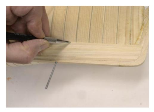
In the next picture the installed plank is being pared back to one-half its width while preserving a fair line forward.
