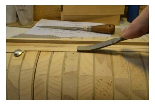
The bottom planking is 4" thick above the garboard. I ripped the planks to 5" to allow for some smoothing out and some finish sanding. Since all of the planking on this model would likely be painted or metal sheathed, I dispensed with pre-painting the edges of the planks and the use of dark glue. The next picture shows some work near midship.
