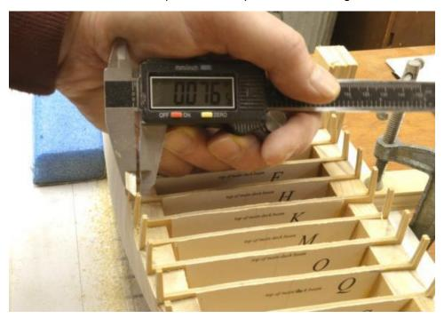
You can see from the reading that they are still oversized somewhat at .076". They would later be faired to the final 6" (.0625") by sanding the insides – but only after some reinforcing outer planking was in place. However, it was necessary at this stage to fair the deck "beams" accurately – as shown in the next photo.
