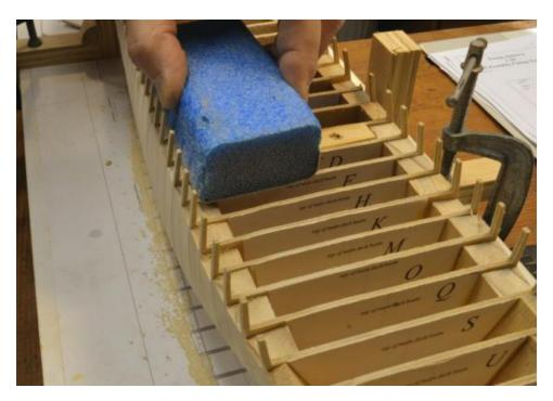
Fairing of the deck was particularly important to avoid waviness in the thin deck planking that would be added later. In the next picture this is being checked during the sanding process using a pine batten.
