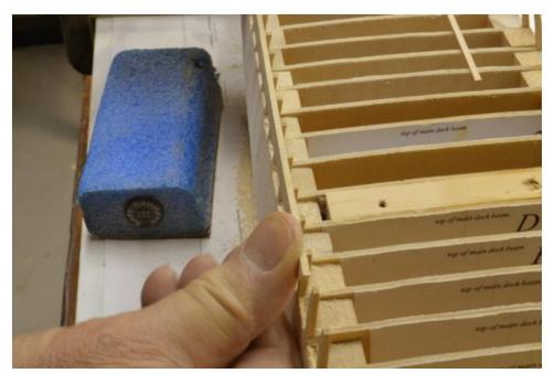
The toptimbers were molded 6" at the top. In the next picture this is being checked with calipers.
