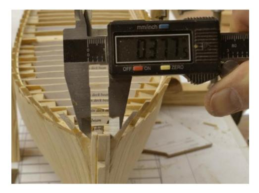
At 1:96 the breadth needs to be 3/8". This precise breadth was obtained by sanding the sides of the members after they were glued in. In the next picture the port knighthead is being glued into place.
