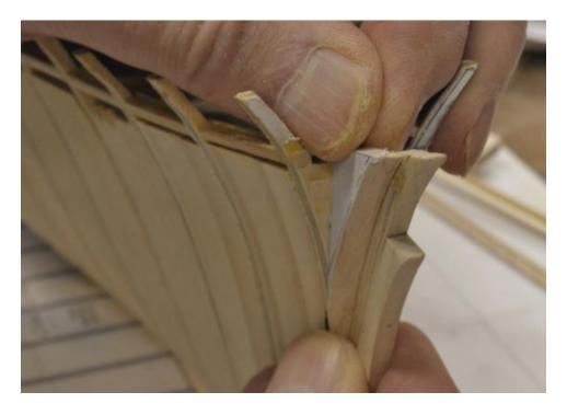
To prepare for this, the pine spacers forward of the first bulkhead were removed by sawing and paring with a straight chisel. These spacers had been installed to protect the forward bulkhead during initial rough fairing of the hull.
