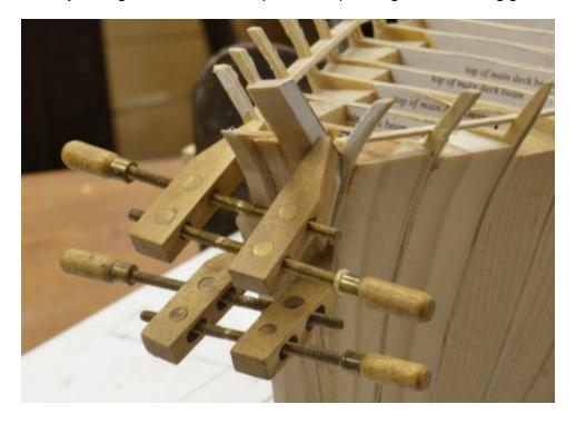
With both knightheads firmly secured they could be faired into the stem rabbet. In the next picture a gouge is being used for this.
