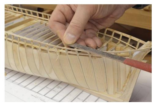
Before sanding the insides of the toptimbers, outboard planking between the main rail and planksheer rail was installed. I will cover fitting of this planking around the stern in a later post. A temporary spacer was used to set the gap that will eventually be filled with the painted main rail. In the next picture the planking down to the planksheer has been installed and the insides of the toptimbers are being faired with a Softsander® pad fitted with 120-grit paper.
