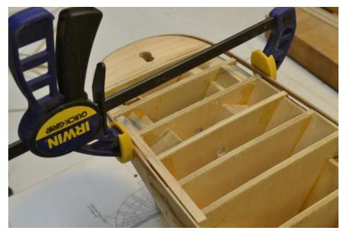
In the next picture, a final check of the height of the stern at the centerline is being checked against the drawing using the height gauge. Last chance to make sure the height is correct.
