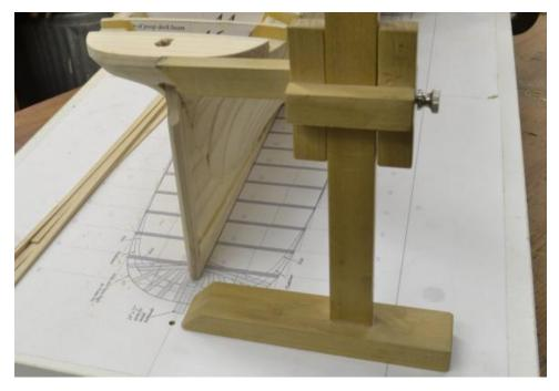
The decking of the poop was flush with the top of the side planking, allowing the fancy rail to cap the side and deck planking. In the next picture a gauge strip of deck plank thickness ( $3 \frac{1}{2}$ ) is being used to check the side planking height as it is glued and pinned in place.
