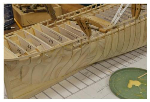
Once the work has proceeded forward of the poop deck and the plywood bulkheads, clamps were used in lieu of the pins as the planks were glued. In the next picture the upper side strakes are complete and the tops of the timbers are being levelled off at the correct height using a fine rasp. This could not be done safely without the upper strake in place.
