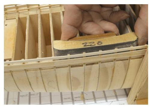
At this stage the upper works were quite strong, the toptimbers sanded smooth and ready for the next step – installation of the inboard parts of the main rail.
