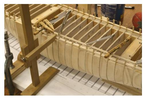
The height gauge was used throughout the installation of this upper strake to ensure an accurate line. The next picture shows some more of the installation of the upper strakes.
