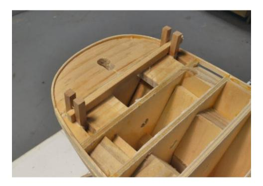
A temporary pine spacer was placed between the bitts to provide correct spacing for the horizontal boomkins. Note the height of the outboard planking around the poop. This will permit the deck planking – specifically the margin plank - to be set flush with the top of these planks. This joint will be covered by the wide "fancy rail" at the top of the side.
