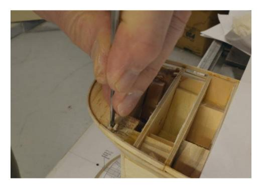
In the next picture the two after bitts of the pair are being glued in. They will be cut down to size and shaped later.
