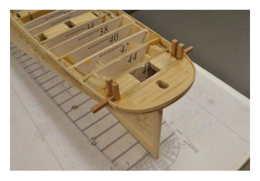
The spacing between the bitts is actually smaller than the size of the boomkins, so they had to be mortised to fit into the allotted space.
