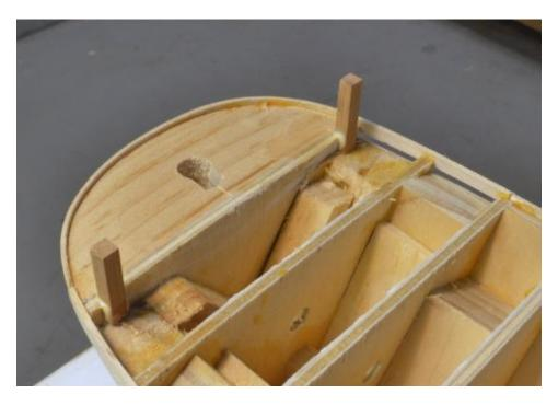
With these in place, wood chocks were fitted to both sides of the installed bits and between bulkheads 48 and 46 – to secure the forward bitts of each pair. The forward bitts are being glued in place in the next picture.
