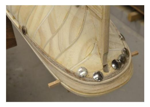
The strake shown above is also highly twisted to conform to the almost horizontal counter at this point. When planks are boiled it is essential that they dry thoroughly and shrink back to normal size. Premature gluing will result in shrinkage gaps between strakes. Waiting for these boiled strakes to dry is time consuming, so other work was done in parallel as shown in the next picture.
