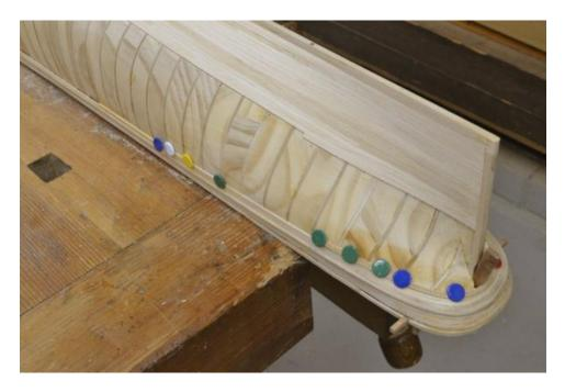
The next picture shows straight planking below the planksheer rail being glued down. The solid soft pine hull allows hammering down of the tacks – making pinning down easy.
