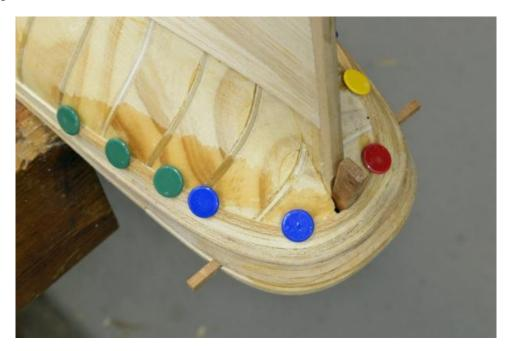
In the next picture this fourth strake is being glued in. The hull is wet from washing off excess glue. The thumbtacks used here have plastic coated heads and are the preferred type. The plastic helps cushion them and reduces damage to the planks. The plastic also prevents wood discoloration caused by wetting uncoated metal heads.
