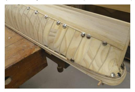
In the above picture the planking is proceeding up from the bottom in parallel with the work at the stern counter. The next picture shows the fourth and final curved stern plank clamped and tacked in placed for drying.
