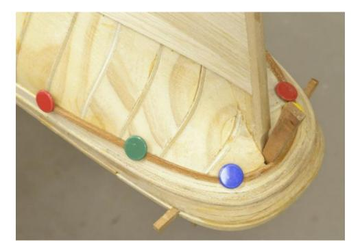
The thumb tacks and the wedge against the sternpost serve to keep this strake tight against its neighbors. In the picture the strakes above have been trimmed by sanding - after drying and before gluing to fit up tightly with the previous planks. They were slightly oversized initially to allow for this final fitting.
