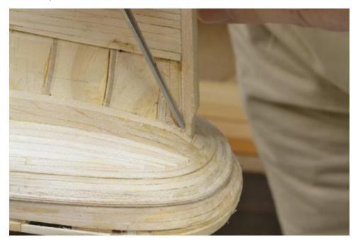
The next picture shows the first plank being fitted into the rabbet. Some curving was necessary as can be seen.
