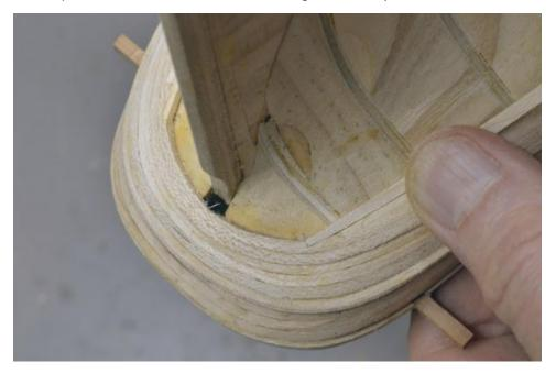
Additional butted planks continued to be added. When the ends of the butts reached an angle of 45 degrees or so, cutting in is eliminated and the ends simply butted into the last curved strake. In the
