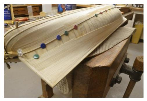
The last picture shows progress at the bow. Fitting the "hooding ends" of the planks into the stem rabbet was simpler than the work at the stern. A heavy clamp was used to make sure these ends were held well into the rabbet and tight against their neighbors.
