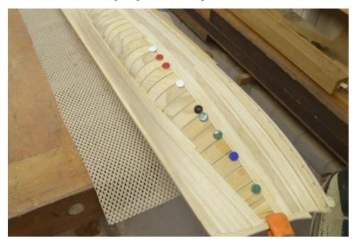
This picture shows that a lot of strake dropping and use of stealers will be needed as the forward (and aft) ends of the hull approach. Completing this planking will be shown in the next post.
