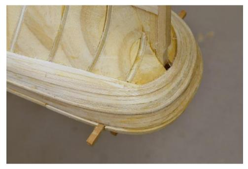
Because the first several of these planks intersect the curved planks at an acute angle, they are "cut in" to the last curved plank to avoid a sharp tapered edge that could not have been caulked. This cutting into the last curved strake is shown in the next picture.
