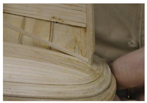
The next picture shows wale planking proceeding downward and the status of the planking from the bottom.
