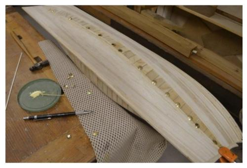
Getting that last space to come out to a 7" opening with parallel sides involved some planning in the placement of the dropped strakes that were necessary both fore and aft. The next picture shows the method I used for setting points where dropped strakes butt into the previous plank.
