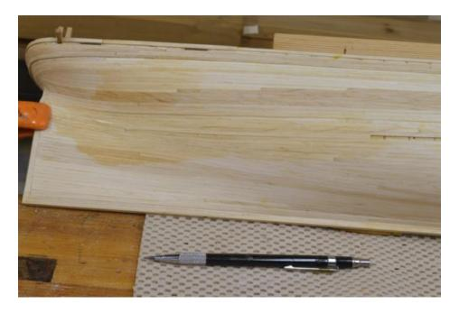
In the next picture that piece is being pressed down into place in a tight fit that required no pinning. A little tapping with a hammer helped.
