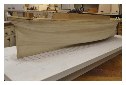
The last picture shows the completed lower planking on the port side down to about midway into the wale. There are 21 strakes of 6" wale planking on the ship. The lower part of the hull was left unplanked on this side to show the method of POB framing used.
