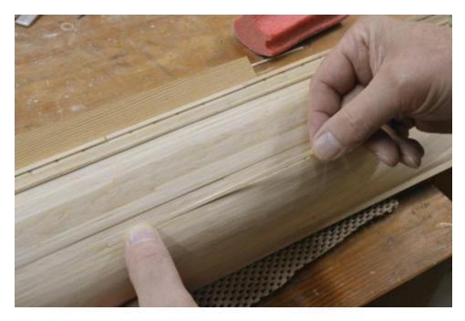
Finally, the completed planking of the bottom on the starboard side.
