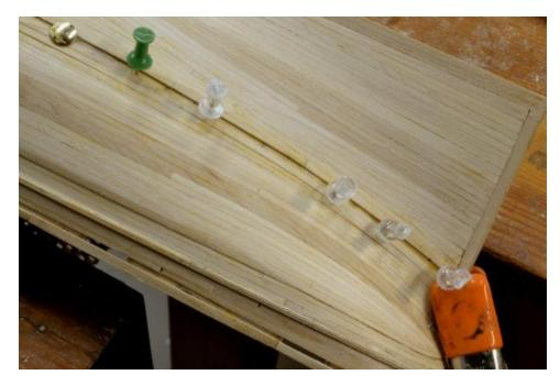
At this stage I was regretting using some slightly darker maple for some of the planks - even though all is intended to be painted. In the next picture this plank has been installed and all that remains is the closing piece near midship.
