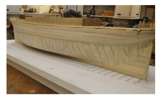
Even though this model initially started out as a demo of the POB framing only, I got a lot of satisfaction in taking it to this further-than-intended stage and eventually went a bit further. Next step was to install the channels....next time.
