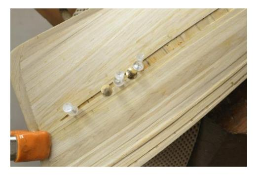
In the picture the narrow space to the left will just accommodate one strake with a taper to half width at the forward end of the opening. The next picture shows the space left for the last plank at the stern.
