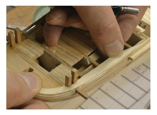
The breadth of the margin plank was then marked out using the compass as shown below. This is a fairly wide plank – wide enough to butt and joggle deck planks into it inside the cap rail that will be installed later.
