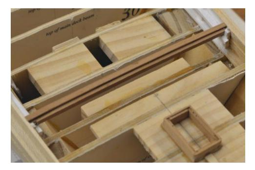
This beam is at station 36, forward of the first poop bulkhead at station 38 to allow some overhang of the forward end of the poop. It was rounded up by a process similar to that used for beams on the larger framed model – but with some differences that I will describe later when the forecastle framing is covered. Rather than cut the rabbet on the top of this beam, a  $3 \frac{1}{2}$ " strip was glued across the top. It overhangs the forward face of the beam by about three inches.
