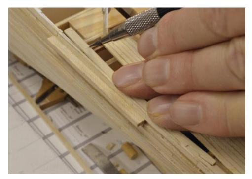
In the last picture the plank is being glued down with the aid of some homemade pin clamps. I will describe these later.
