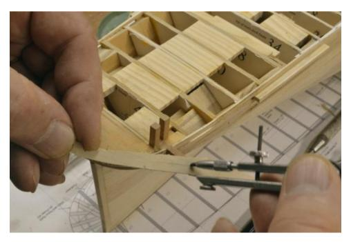
Again, to avoid breakage at the curved end of this piece when sawing, it and the piece for the opposite side have been pasted to plywood. The curve of the starboard piece is being cut in the next picture.
