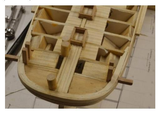
The fit against the outside planking does not have to be perfect, since it will be covered by the capping fancy rail. This picture also shows hatch coamings and decking that I worked on concurrently. This will be covered later.
