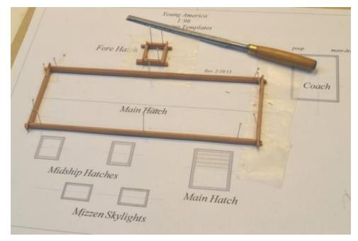
The hatchways for the POB model were made in exactly the same way as those on the larger framed model. I described this process in the build log for the other model and more thoroughly in the book. In the next picture a dovetailed lap joint at the corner of the main deck cabin coaming is being fitted.
