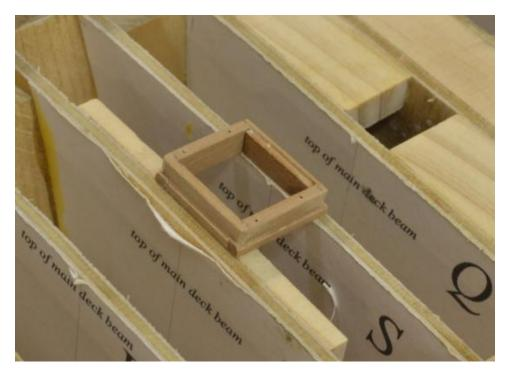
To support the ends of the planks forward of this framing, another supplementary member was need and later installed. In the next picture the coamings on the poop deck have been installed and planking has begun starting with the central plank.
