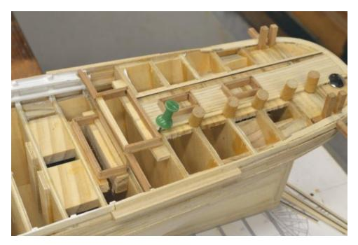
Note that the cap on the breast beam was cut out to fit the aft section of the coach framing. The lower part of this coaming is shown installed on the main deck. These two assemblies had to be carefully aligned so the side walls of the coach would fit neatly – and vertically. Another view of this is shown in the next picture.
