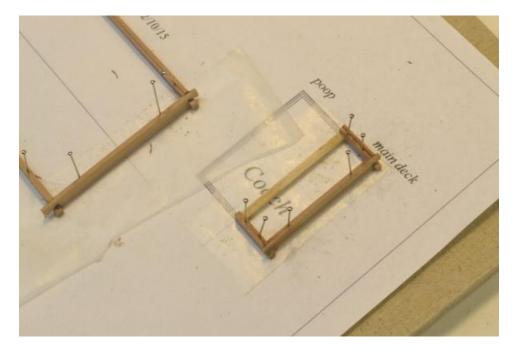
A reinforcing strut was glued into this assembly to maintain the correct width. The next picture shows a finished hatchway installed on a bulkhead and on to one of the supplementary pine members described in an earlier post.
