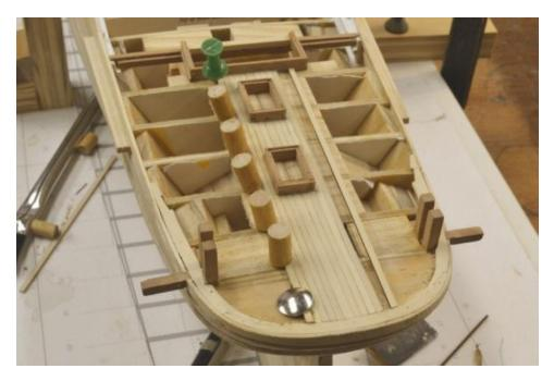
This picture shows the first version of the pin clamps I used to hold down the glued planks on this model. I will discuss the improved final version of these in the next part.
