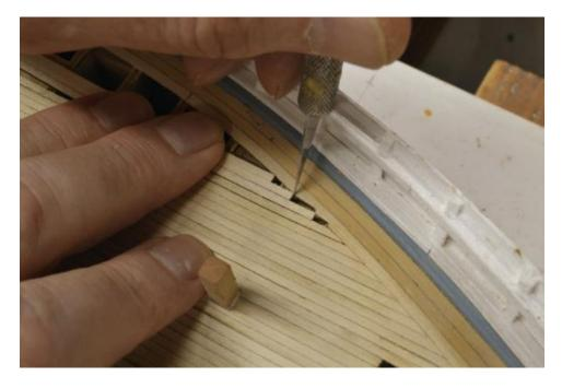
These marks define the cutting in points. At each of these a knife or chisel cut was made into the margin plank perpendicular to the deck plank ends and one-half of the plank width. The shapes of the required plank tapers can be seen in this picture. Note that the joints get longer going aft, as the curvature of the side becomes less.
