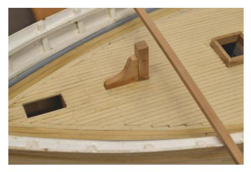
In this picture the Samson post knee has been installed and the breast beam made and laid across the bulwarks. The bowsprit opening has been enlarged to the required 36" width. In the next picture the main deck planking is approaching completion.
