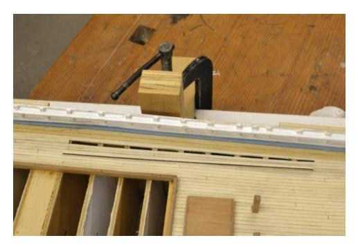
Except for the uncovered hatches, the crude POB framing under the deck was now completely covered – a moment I was waiting for. In the next picture the last plank is in.
