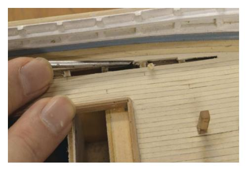
I cut the joints while there is sufficient space for the chiseling - before the adjacent planks were installed. The chisel is a long, straight, model-sized paring chisel – one of my most frequently used and most essential tools. Directions for making these chisels were included in *Naiad Volume I*. In the next picture a shaped plank end is being fit into its joint.
