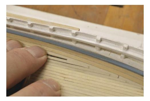
For best visual results the pared side of these planks should be painted like the inner edges – to show the caulk line. I did not do the on this demo model – relying solely on the dark glue to highlight the joint.
