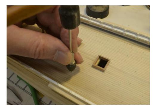
For this work a length of syringe was held in a pin vise that could then be lightly tapped with a hammer. I was very careful to emboss all fastenings directly over bulkheads or other under-deck supports to avoid the possibility of breaking the planks. I used a light pencil line across the deck for each row, then alternated fastenings on either side of the line.
