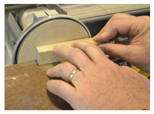
Using a compass the depth of the forecastle beams was then drawn along the curve. A blank that will be sliced into several beams was then cut off along this line, allowing some excess for sanding.
