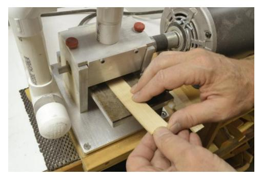
The thickness sander does a great job with this. The depth is uniform and parallel to the top face. It is also very fast. Without a thickness sander, I would have cut very close the line with the scroll saw, then sanded the underside by hand – not too arduous a task. The individual beams were then ripped off –top side down! – on the circular saw as shown in the next picture.
