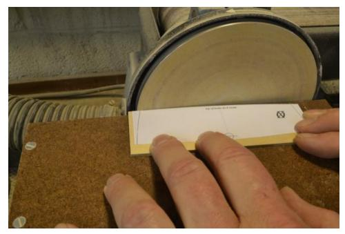
Since the round up radius is the same for every frame and every deck, any one of the patterns could be used. The template was then used to trace the round up on to a piece of maple. The curve was then sanded on to this piece as shown below.
