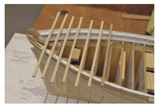
As can be seen, I made these beams long before they were needed - before the planking of the main deck. Cutting and fitting of the beams will be described in the next part.
