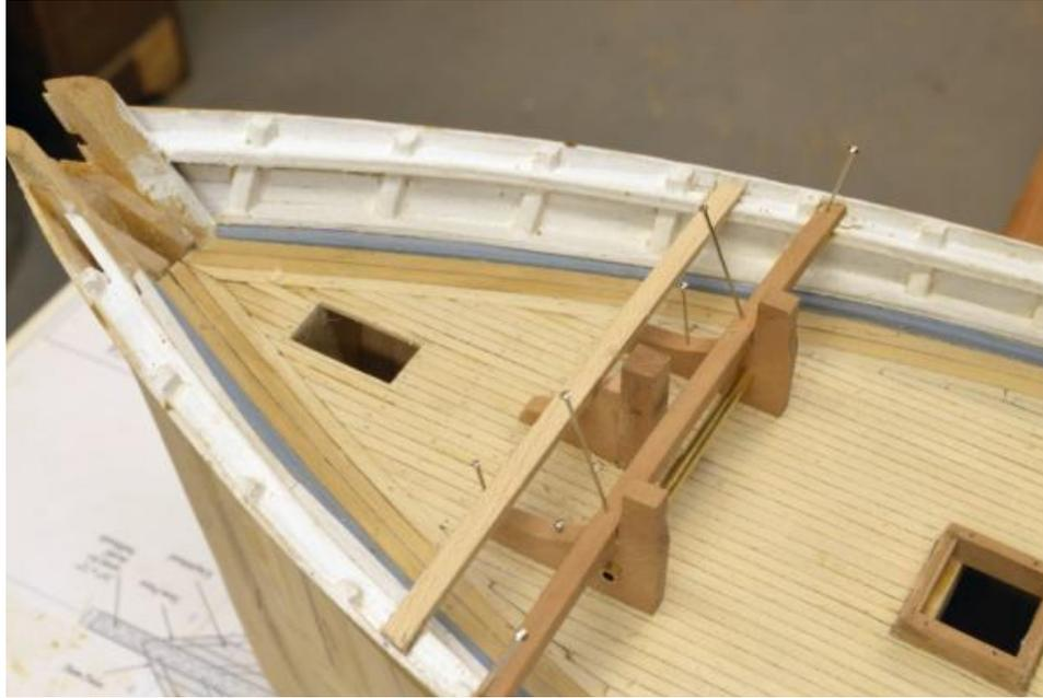
In this picture the carrick bits are pinned in place. They have been positioned with a temporary windlass axle installed so they would be aligned when pinned. The height of this axle was set using a gauge block cut to the correct height when the bottoms of the carrick bits were trimmed before setting. In the next picture the axle has been removed and the bits glued to the deck.
