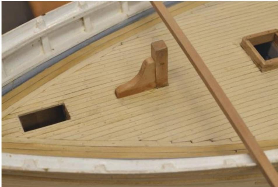
On this model the bowsprit will step on the plywood bulkhead at the aft side of the opening. A dowel into holes in both the bowsprit and the bulkhead would probably be the simplest method. Next, the carrick bits that will support the windlass shaft were cut out. In the next picture, blanks for two bits were pasted together with one pattern and are about to be cut out on the scroll saw.
