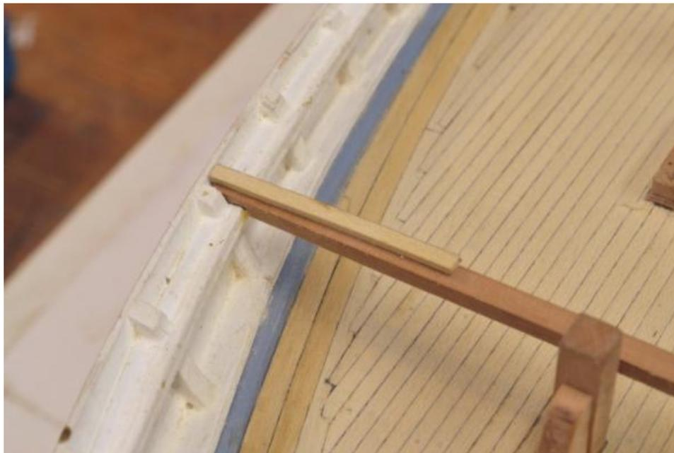
The deck planking needs to be flush with the top of the side. The height along the top of the side was well checked much earlier. I set the deck beams on the top of the main rail, since this is at a
