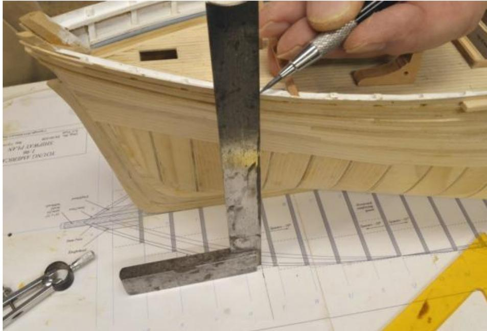
The line drawn at the beam location can be seen at the base of the square. With the first two beams positioned, the carrick bits and the Samson post knee could be trimmed to provide support for the beams. All these parts have been fitted in the next picture.
