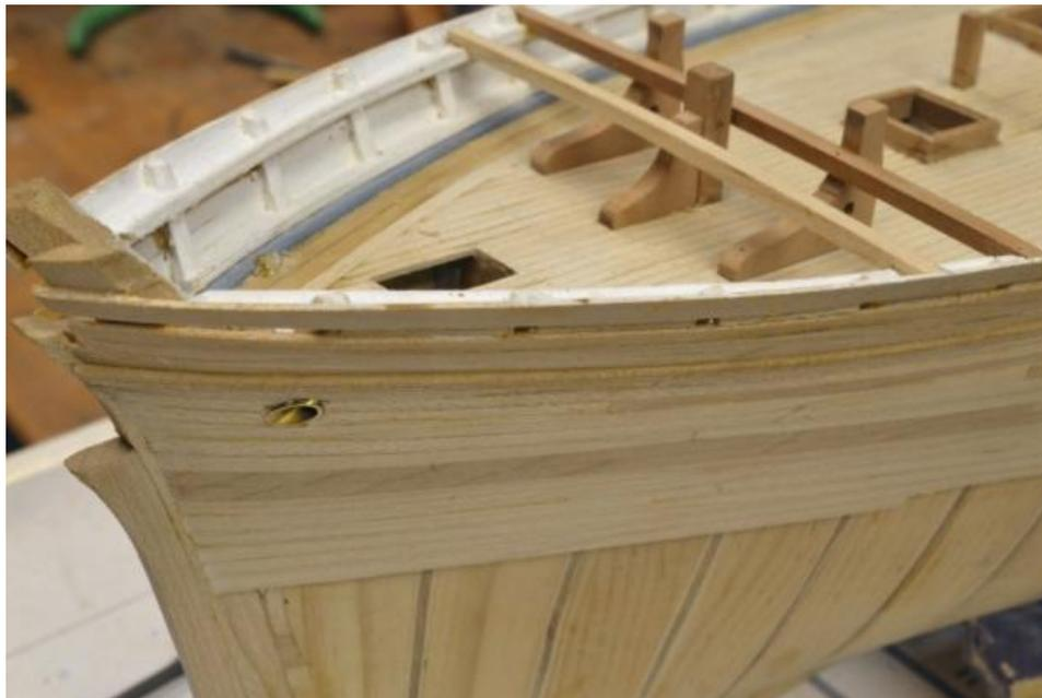
All four hawse holes were installed in this manner. The linings were the filed off flush on the outside. Work on the forecastle deck will continue in the next part.
