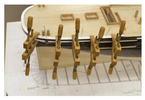
In the next picture the rail on the opposite side is being installed.
