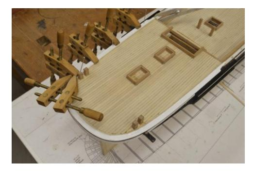
In the picture the leftmost clamp is closing the scarph joint in the rail. Note also that these rail sections end at the forward edge of the breast beam. At this point the rail thins down in width, so the next sections along the main deck will be narrower, but the outside line of the rail will be flush.
