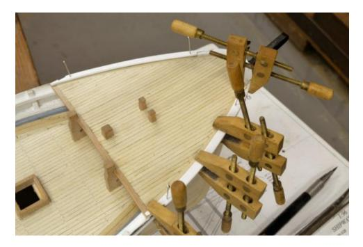
Note the use of a screw clamp to close the joint to the forward section. The next step is shown in the last picture.
