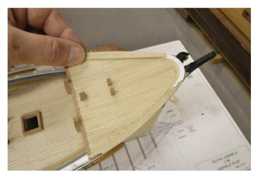
The joints were then formed on these, the edges rounded, and the pieces painted before installation. The starboard piece is being glued in the next picture.
