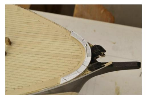
A template made from one of the pdf drawings was used, since the outer shape could not be traced as was done on the stern. The joints were then formed, the inside (only) edge rounded by sanding, and the piece painted. It is shown pinned in place below.
