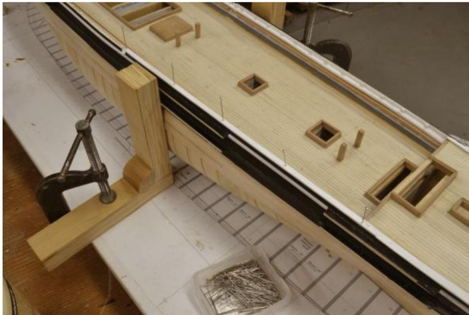
The pins are placed in the toptimbers. The holes will later be filled with copper wire bolts to reinforce the connection and fill the holes.
