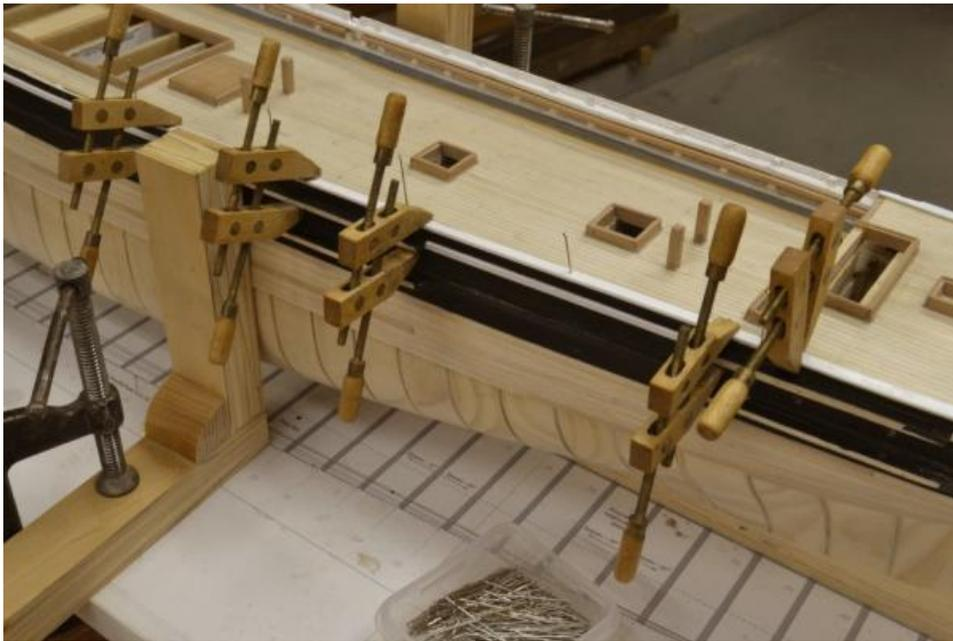
At this stage all the excess glue was washed off with water. The next three pictures repeat the process on a forward section of the starboard rail.
