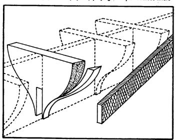
you have obtained the necessary angle of the frame edges. Repeat this all the way down, then do the same in the direction of the stern until you are satisfied that you have got all the angles right. Do the same for the other side of the ship.
