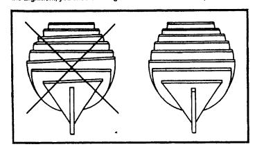
wood glue, reset the frames into position again as before and leave this framework to completely dry out before going on. You must leave this in such a position so as not to disturb the lay of the timber frames. Prop it up between two books or clamp into position with suitable clamps. You will have noted that the top and bottom edges of the frame No. 14 will have to be chamferred down so as to fit flush into position.
