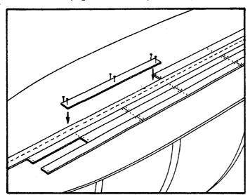
me to do so, you can add a touch of realism to this job by tinting the edges of each plank with a little ink so as to represent the caulking of the deck. The choice is yours, because to do this needs a deal of patience. We have seen for example, how one of our clients once used black thread between each plank to represent this caulking, and it was very effective. Although we are not recommending that you go to such lengths, it does show the ingenuity of some model-makers
