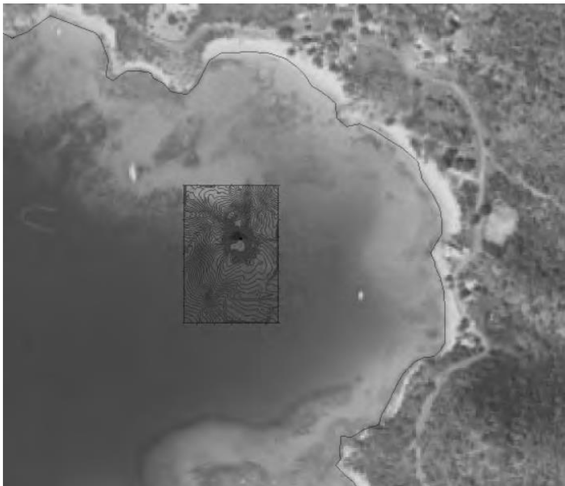
Figure 19: Magnetic survey of the HMS Santa Monica (Rodgers, et al., 2002).
